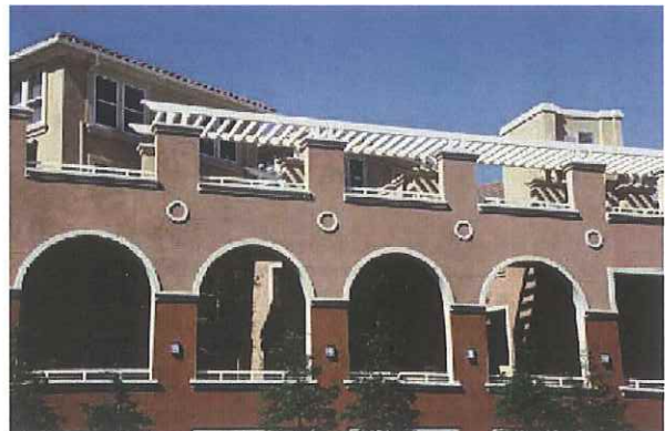
Architectural features that add human scale and provide usable outdoor space, such as balconies, loggias, and trellises, are recommended.
