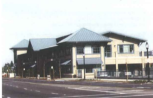
Pitched roofs may exceed height limits if gable or other non-shed roof types are used.
